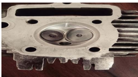
Figure 9 Cylinder Head Machined with Grooves
